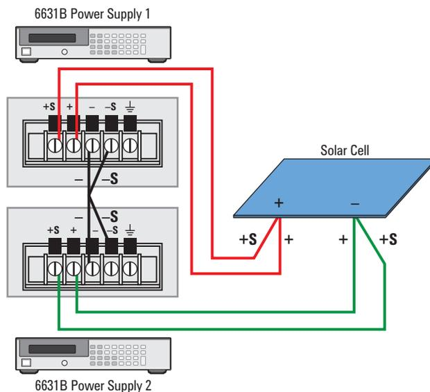
**Figure 2. A pair of two-quadrant DC sources connected in anti-series**
