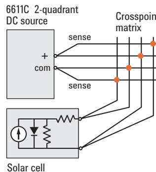
Figure 1B. Solar cell electrical characterization test setup configured to capture the reverse bias electrical characterization of a solar cell
