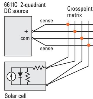
Figure 1A. Solar cell electrical characterization test setup configured to capture I-V curve of a solar cell
