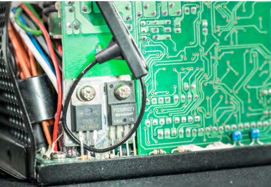
Figure 8. A Rogowski probe tip wrapped around a component.
